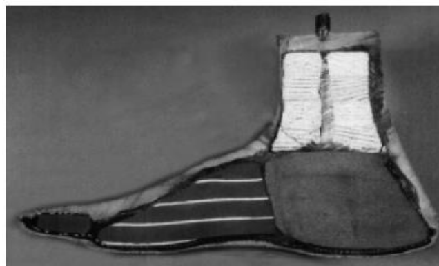
Figure 6: A sagittal section of a Jaipur foot (Arya et al. , 2008).
